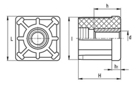
$\begin{array}{lll} d & = M10 \\ h & = 10 \\ H & = 45 \\ h1 & = 10 \\ Internal tube size = 45.0 \\ I & = 45.0 \\ L & = 50 \\ \end{array}$
